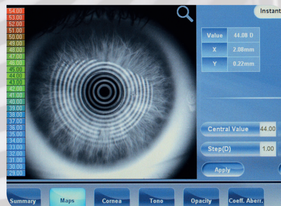
Full automated topographer, placido rings technology
