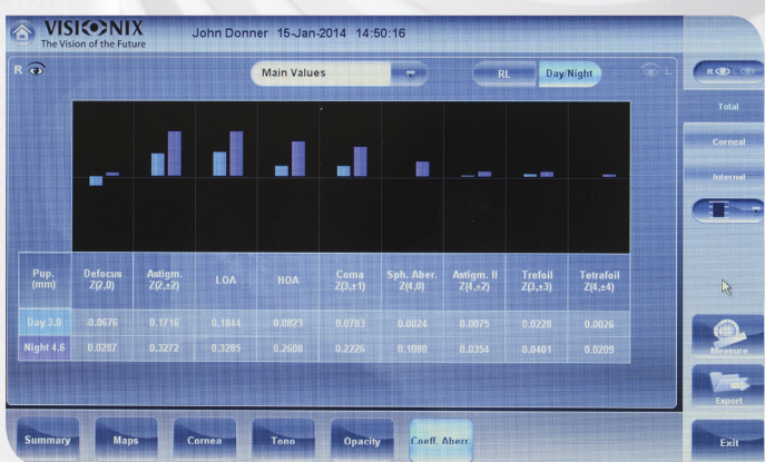
Full automated aberrometer PSF and Zernike analysis
